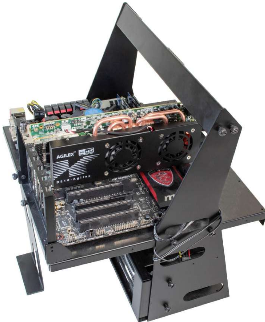
Figure 8-4 FPGA board installation on PC
