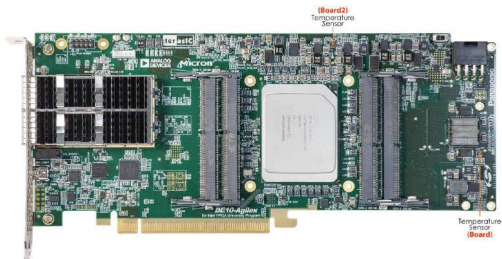
Figure 10-10 Location of the board's ambient temperature
