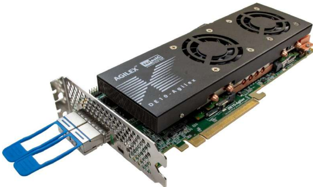
Figure 9-9 Setup QSFP28 or QSFPDD loopback fixture
