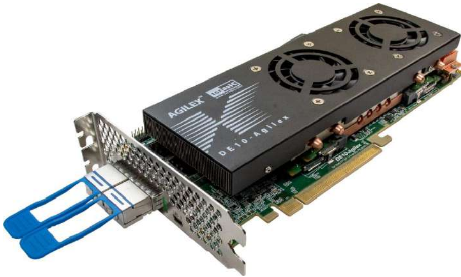
Figure 9-14 Setup QSFP28 or QSFPDD loopback fixture
