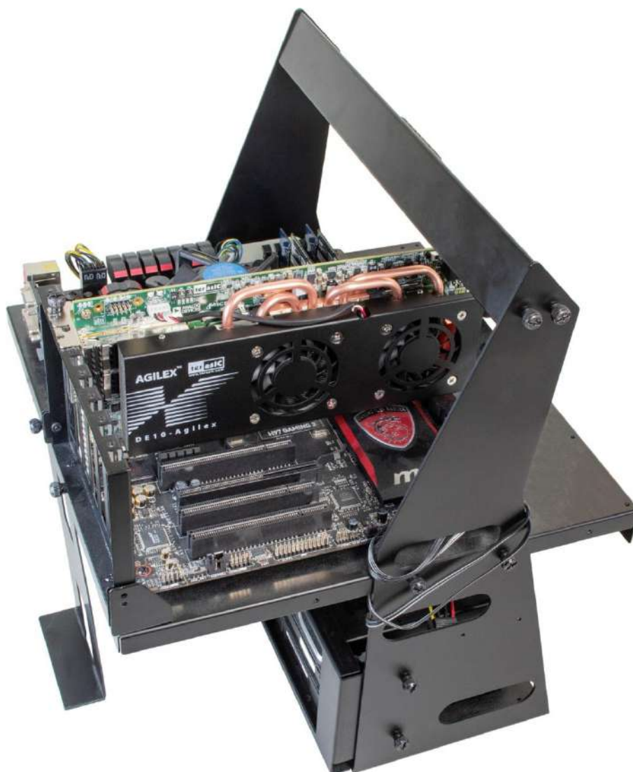
Figure 7-9 FPGA board installation on PC
