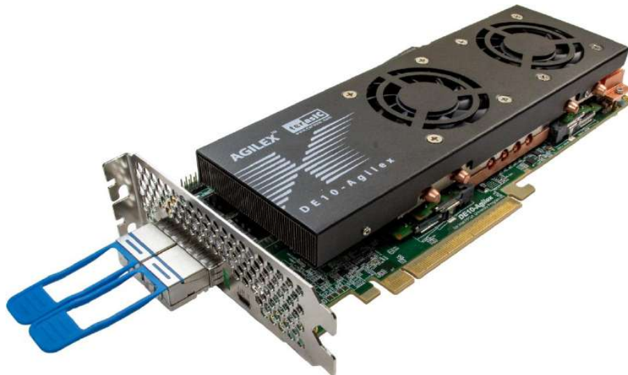
Figure 9-2 QSPF-DD Transceiver Loopback Test in Progress
