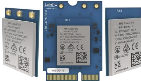
Introducing the first of the Sona™ Wi-Fi 6/6E product line from Laird Connectivity, the IF573, based upon Infineon's leading AIROC™ CYW55573 chipset. A truly robust industrial IoT module: one that's rugged, small, globally certified, has reliable connectivity, and is easy to integrate.
