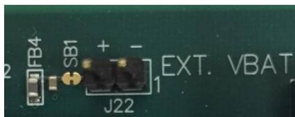
Figure 5: External VBAT power connector
