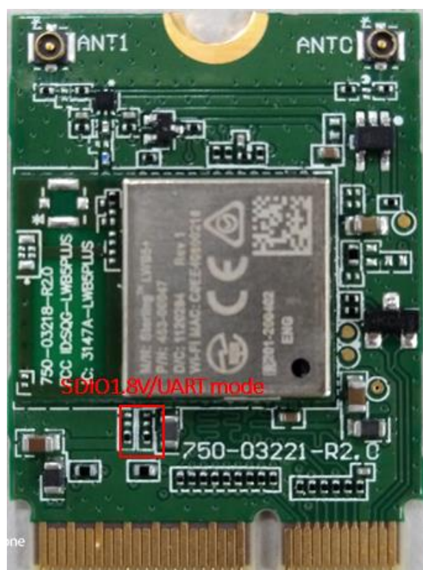
Figure 2: Hardware strapping for the LWB5+ M.2 SDIO/UART variant
