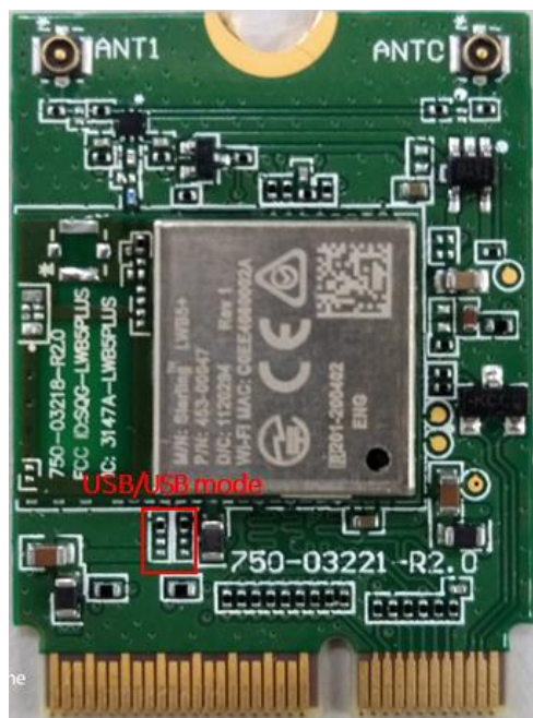
Figure 4: Hardware strapping for the LWB5+ M.2 USB/USB variant
