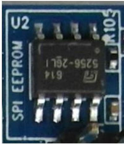
Figure 17: SPI EEPROM schematic and PCB
