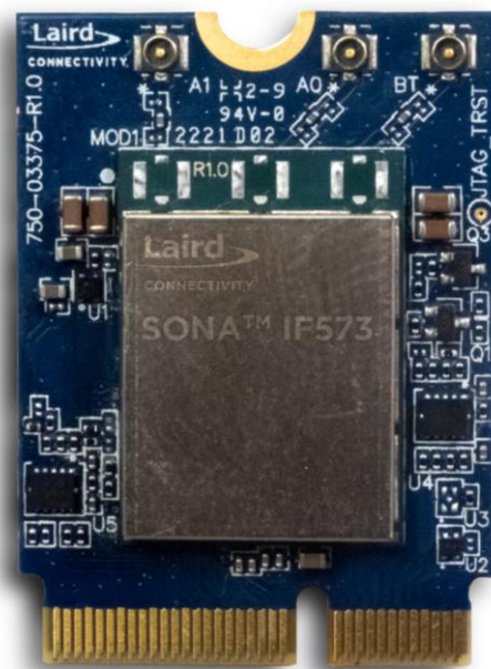
Figure 2: Sona IF573 M.2 Module
