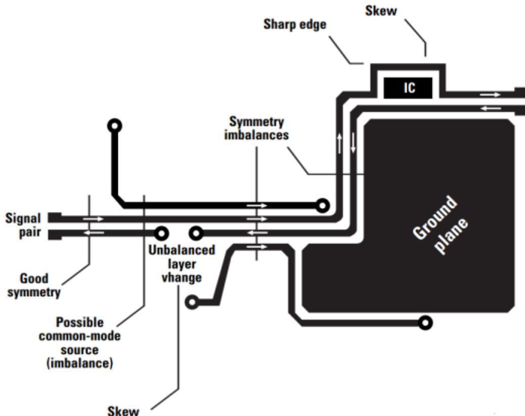
A conductor that carries current requires an opposite mirror current to return through some part of the system. This return current path will be the path of least resistance. For high-speed signals, the return current path will be the path of least inductance.
