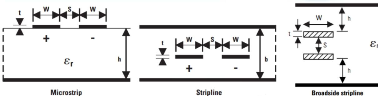
Use controlled impedance PCB traces that match the differential impedance of your transmission medium (e.g., cable) and termination resistor. Route the differential pair traces as close together as possible (use the minimum spacing "S" specified by your PCB vendor) and as soon as they leave the sensor. This helps to eliminate reflections and ensures that noise is coupled as common-mode.
