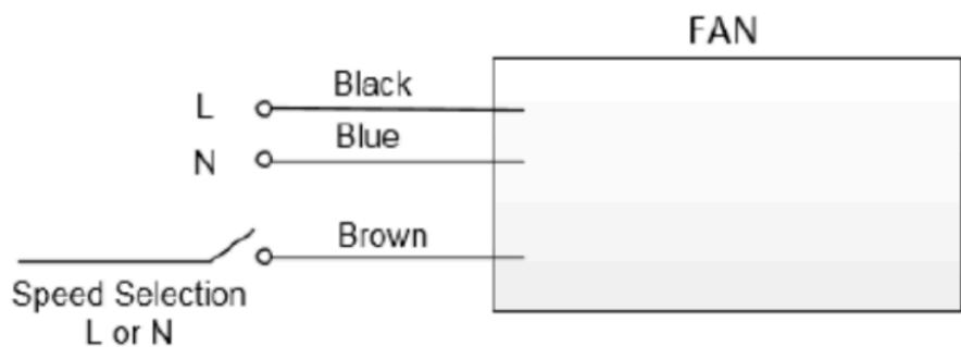
When the Black or Blue wire connect to Brown line, the Fan speed will switch to low speed mode.
