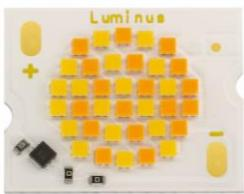
*Dim-to-Warm modules replicate the behavior of traditional bulb technology by changing CCT from 3000K to 1800K or from 4000K to 2700K as they are being dimmed. Luminus is the only LED supplier offering a choice of dimming curves, with either halogen-like or linear-style effects available across all four LES options and both CCT ranges. These UL listed modules have 9000-hour LM-80 data at 250mA per LED with L90>36k hours to enable DLC premium.*
