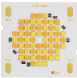
Luminus Dynamic CCT Modules offer a choice of 9, 14, 18, and 22mm LES options, all with two independent channels (warm and cool) to deliver CCTs ranging from 6500K to 2700K or from 4000K to 1800K. This wide range of options provides luminaire makers with flexibility in designing human centric lightning applications with independent CCT and dimming control. These UL listed modules have 9000-hour LM-80 data at 250mA per LED with L<sub>90</sub>>36k hours to enable DLC premium.
