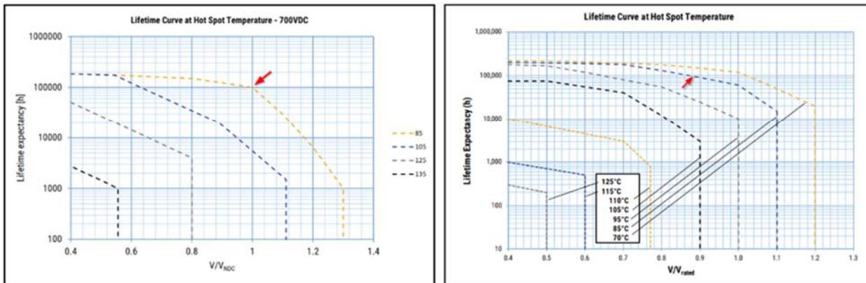
Another example of this lessened need for voltage derating at high temperatures is shown in the below comparison plot versus the new DC-Link solution. In this example, the C4AK technology requires less voltage derating beyond the 85°C hot-spot than C4AQ-P technology. C4AQ-P is capable of reaching a 125°C hot spot temperature. This capability translates into higher voltage capability at high hot-spot temperatures and the possibility of using fewer capacitors (miniaturization).
