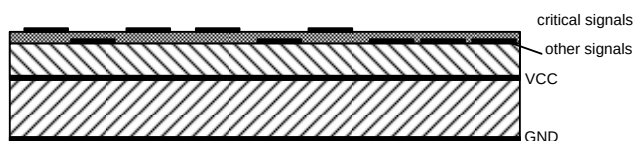
Figure 22. Wrong: VCC and GND planes are too far apart
