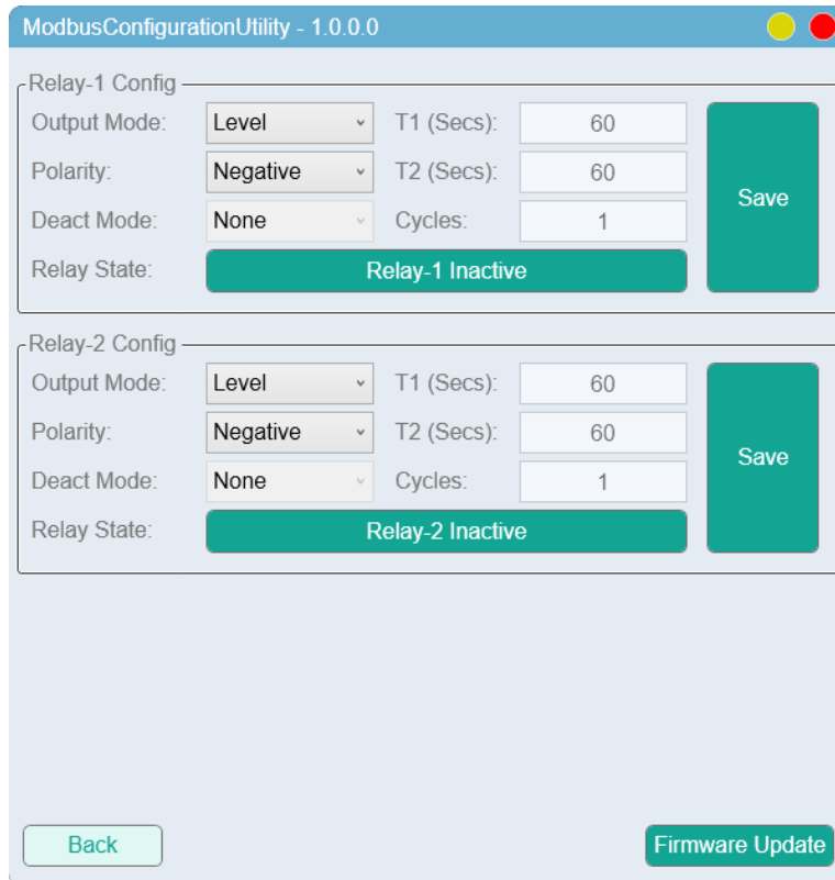
Figure 17 - Modbus 2CH Relay Control Window
