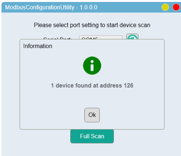
Figure 11 - Modbus Configuration Utility After Scan Message
