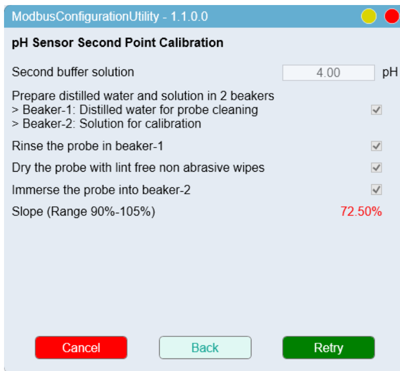
Figure 46 - Modbus pH Sensor Second Point Calibration Failed Reading
