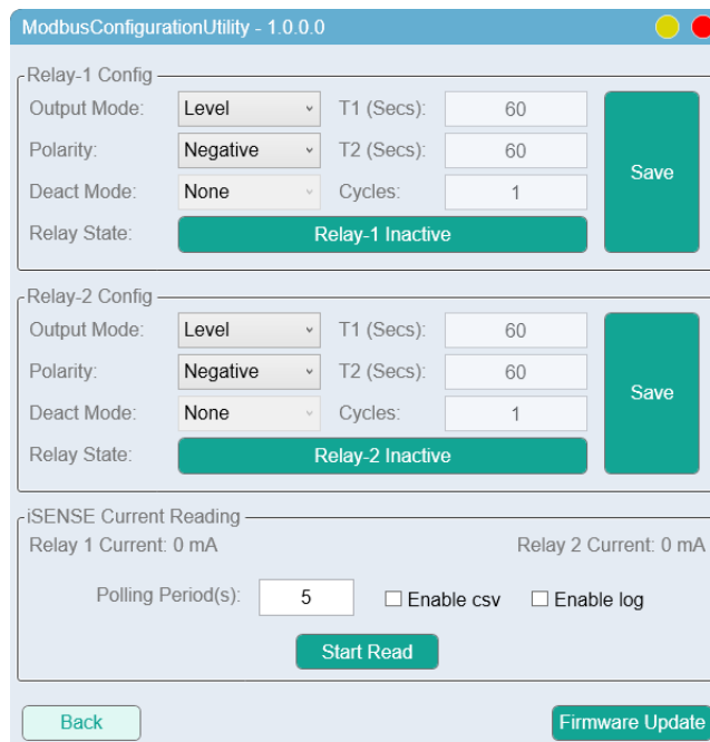
Figure 18 - Modbus 2CH Relay + iSENSE Control Window
