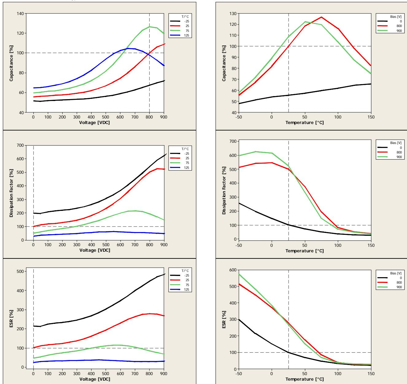
Typical capacitance values as a function of voltage  $V_R = 900$  V
