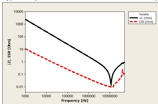
$V_{DC} = 0$  V,  $V_{AC} = 0.5$  V<sub>RMS</sub>,  $T_{device} = 25$  °CTypical permissible current as a function of frequency  $V_R = 900$  V
