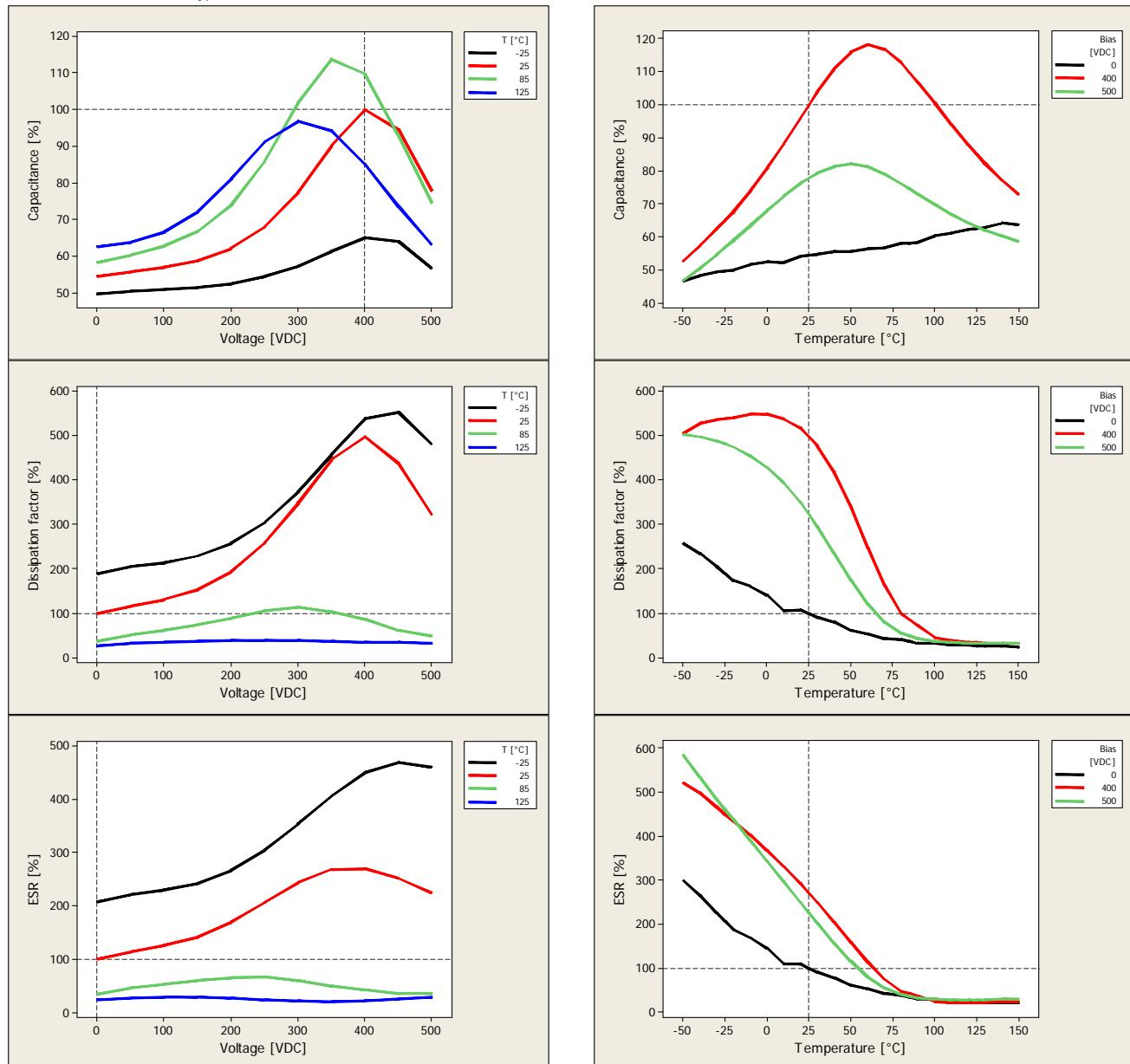
Typical capacitance values as a function of voltage  $V_R = 500$  V
