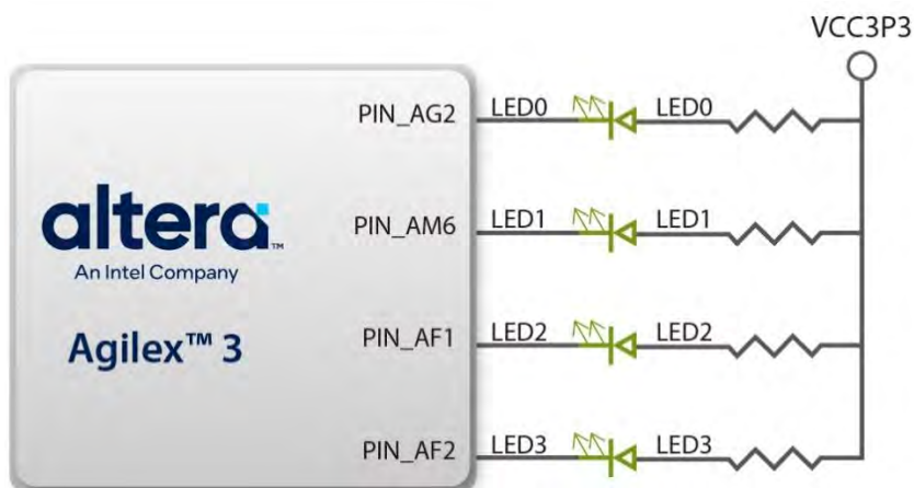
Figure 3-14 Connections between the LEDs and the Agilex 3 FPGA
