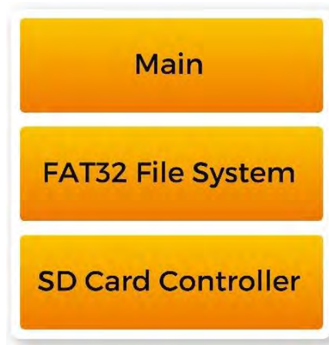
Figure 4-5 Nios V Software Stack of the SD Card Demonstration
