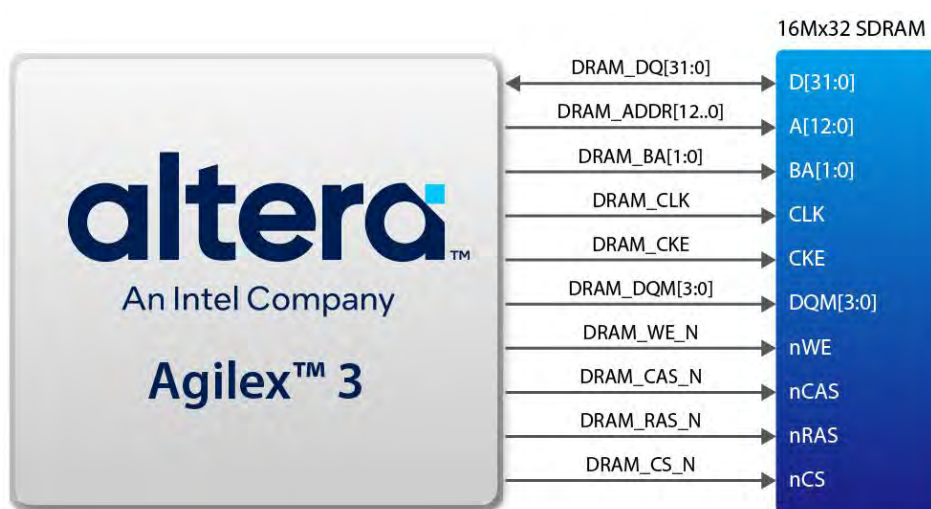
Figure 3-19 Connections between the FPGA and SDRAM
