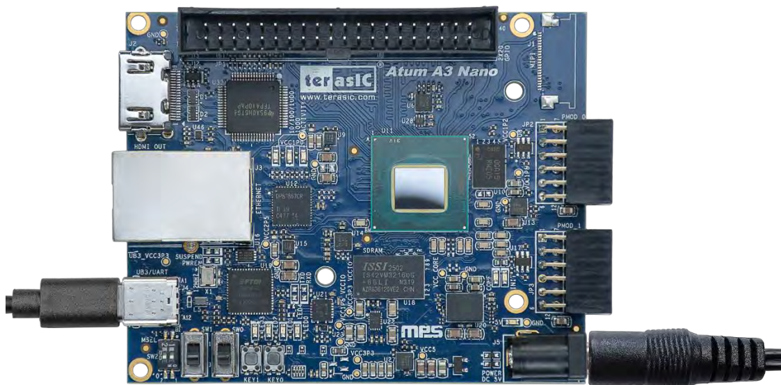
Figure 5-3 Power and USB cable connection for the board
