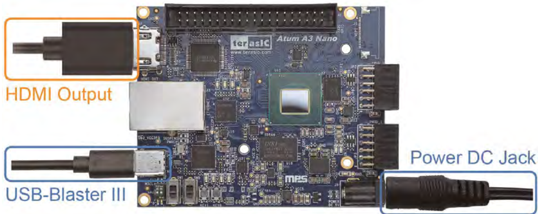
Figure 3-2 USB Blaster III, HDMI and Power Jack on Atum A3 Nano board
