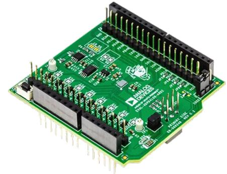
The EVAL-ADPD410x-ARDZ Breakout Boards can also be adapted for other evaluation platforms including the EVAL-ADPD4100Z-PPG, optimized for photoplethysmograph applications, and the reference design CN0503, optimized for optical liquid analysis applications (colorimetry, turbidity, fluorescence). This helps in meeting specific application requirements, as well as for the ground-up development of different applications.
