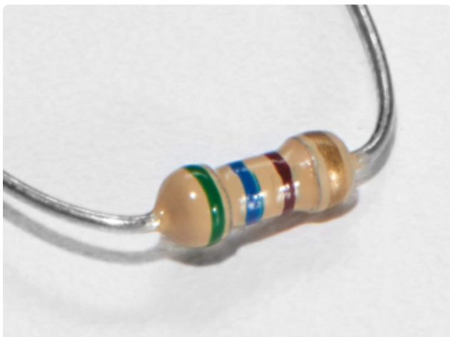
560 Ohm Resistor Colors: Green > Blue > Brown
