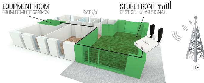
Site survey using the included battery will help you locate the best signal strength to send back to your router while remotely powering using the included PoE injector.
