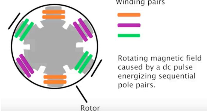
EC motors are controlled by external or onboard electronics that convert the incoming AC power signal to the DC voltage needed by the motor. The electronic circuitry performs the function of the mechanical commutation that switches the direction of the
