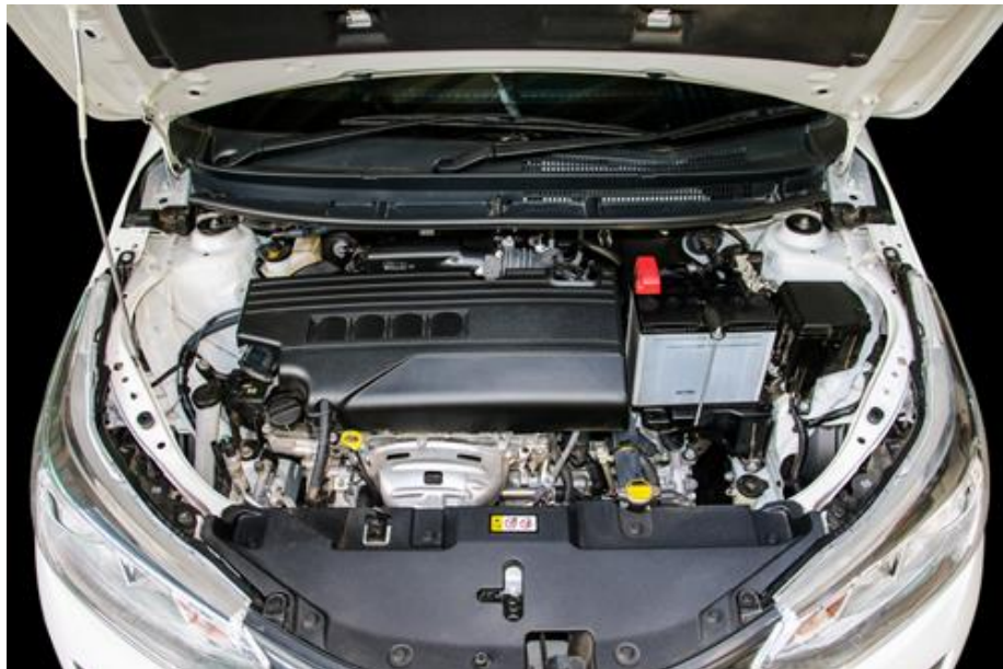
Figure 1. The Lead-Acid Battery Powers the ICE Car Electronics
