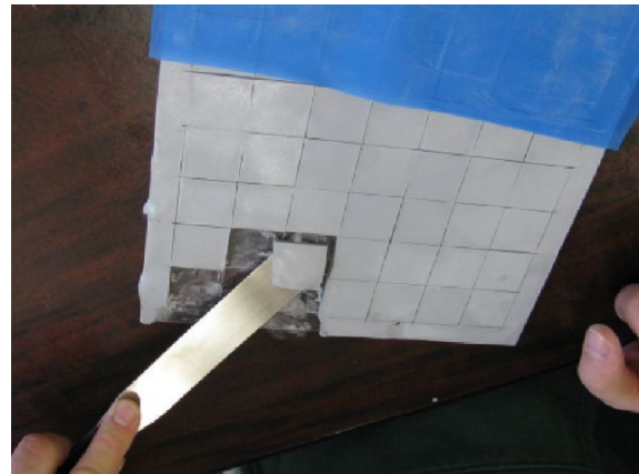
Figure 8. A tool (i.e. spatula) is strongly suggested to remove converted parts.
