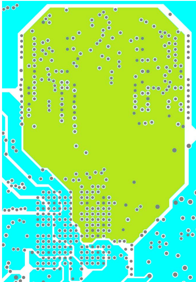
Figure 3-4. SAMA5D2-XULT Layer 5 (VDD)
