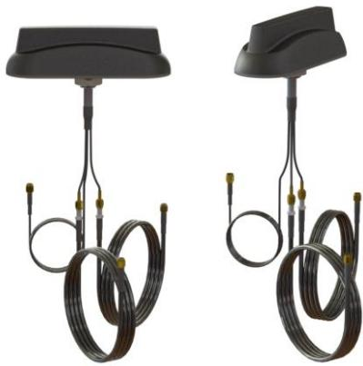
The Gar VFT69383x11JN multiport/multiband antenna provides an excellent solution for public safety, transportation, and aftermarket fleet applications. Configured for one-port operation over the 3G/4G/5G/ISM/CBRS bands and one-port operation over the low/high frequency Wi-Fi bands. An additional third port provides an active antenna for enabling GNSS global navigation services.
