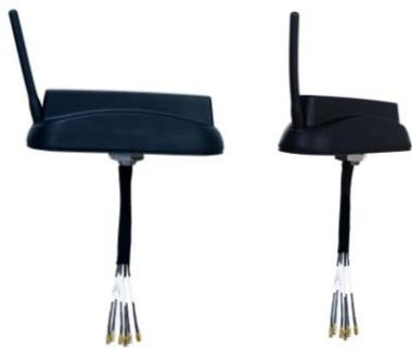
The Barracuda VFH69383B23JW multiport/multiband antenna provides an excellent solution for Public Safety, Transportation and Aftermarket Fleet applications. Configured for 2-port MIMO operation over the 3G/4G/ISM/CBRS bands and 3-port MIMO operation over the low//high frequency Wi-Fi bands. An additional 6<sup>th</sup> port provides an active antenna for enabling GNSS global navigation services.
