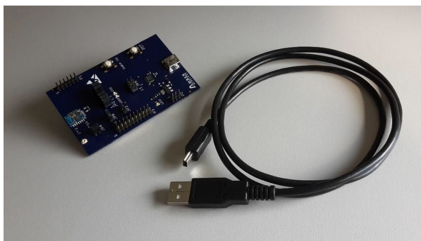
Figure 2: USB cable and evaluation board of the Proteus-I and Proteus-II radio module
