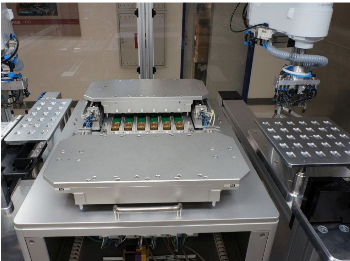
Figure 9: Automatic test equipment for module test
