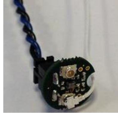
Figure 18. MicroFC–10020–SMT Detector Mounted at the Centre of the Readout Board
