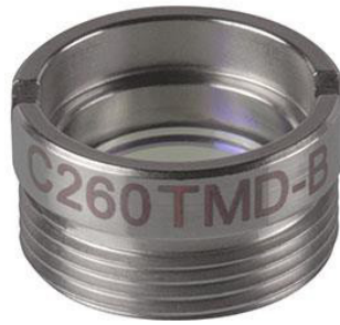
Figure 4. C260TMD-B f = 15.29 mm, NA = 0.16, Mounted Geltech Aspheric Lens, AR: 600–1050 nm
