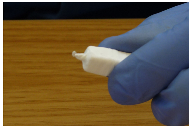
Figure 8. The End will Look Like This. The Point can be Trimmed Off if Desired. The Wrapped Crystal is Now Ready for Use
