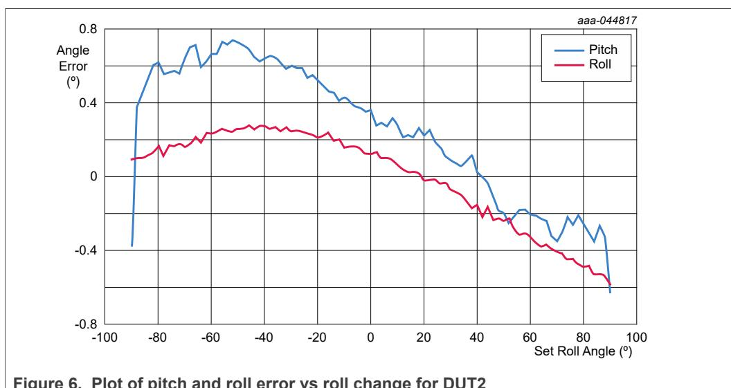
Figure 6. Plot of pitch and roll error vs roll change for DUT2
