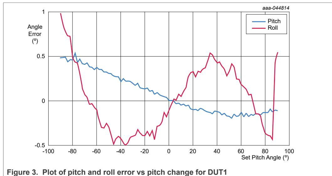
Figure 3. Plot of pitch and roll error vs pitch change for DUT1
