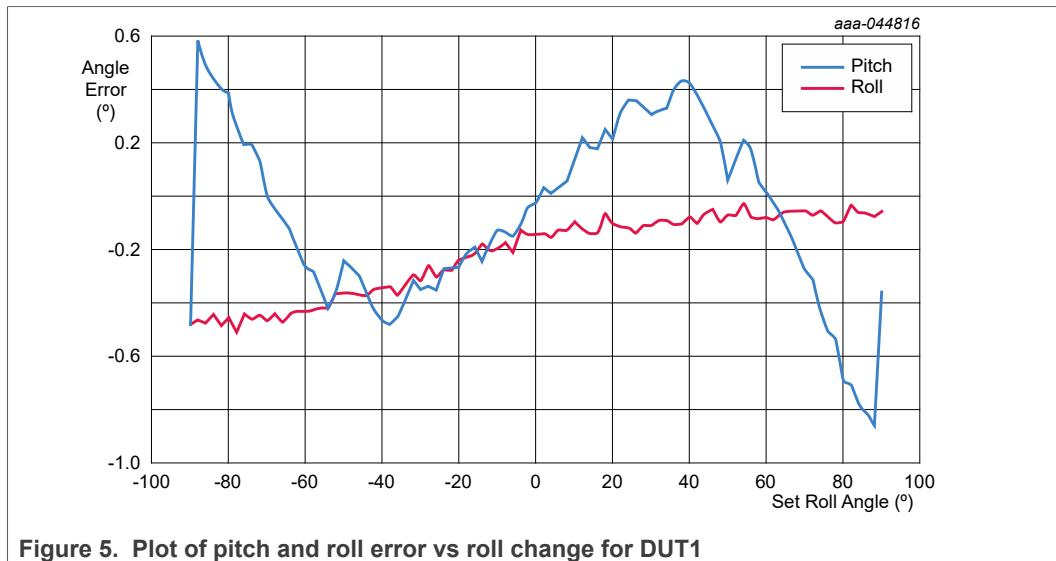
Figure 5. Plot of pitch and roll error vs roll change for DUT1
