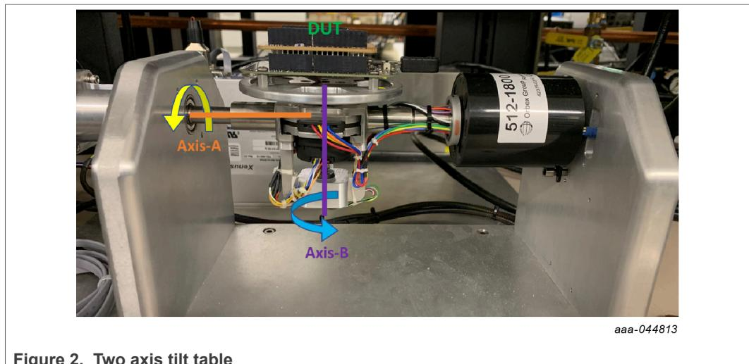
**Figure 2. Two axis tilt table**
