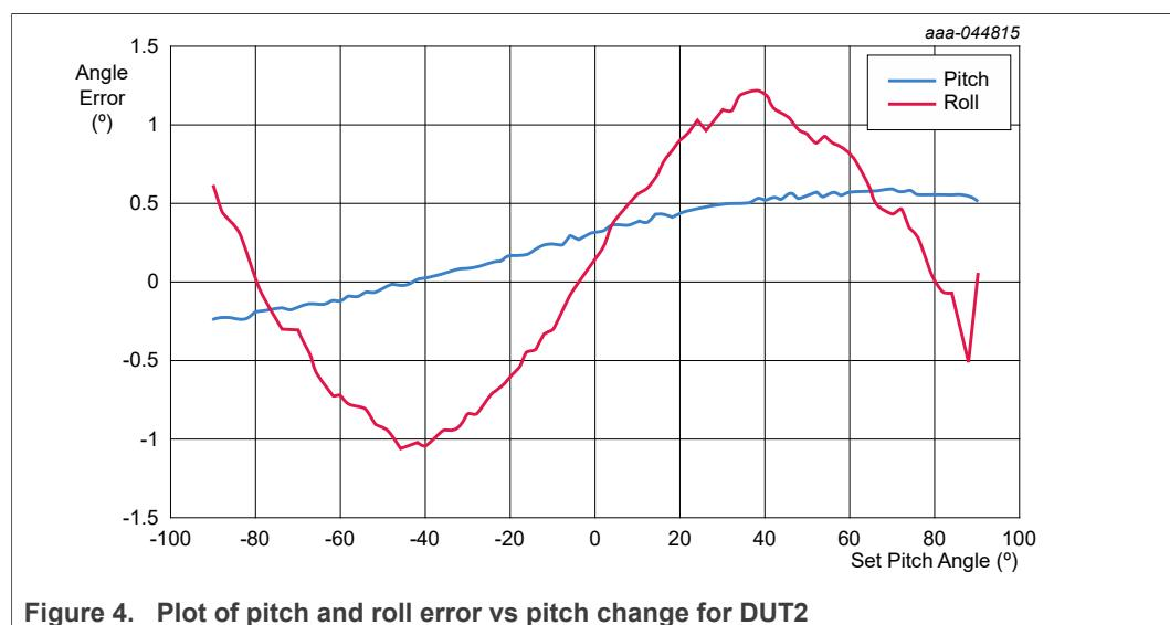
Figure 4. Plot of pitch and roll error vs pitch change for DUT2
