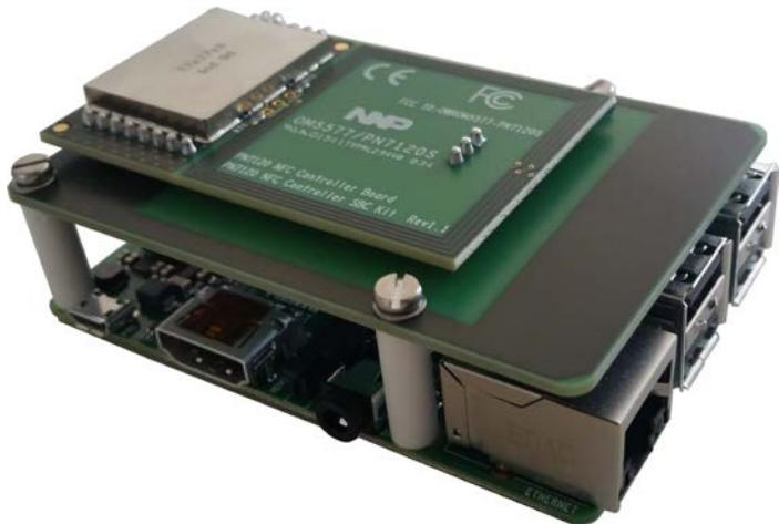
Fig 4. OM5577/PN7120S demo kit stacked on Raspberry Pi 2 board
