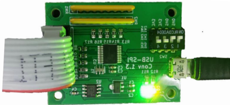
Figure 8: HEDS-9930(E2/E2L)PRGEVB USB-SPI Programming Kit Detected by the AEDR-9930_Gateway.exe Program
