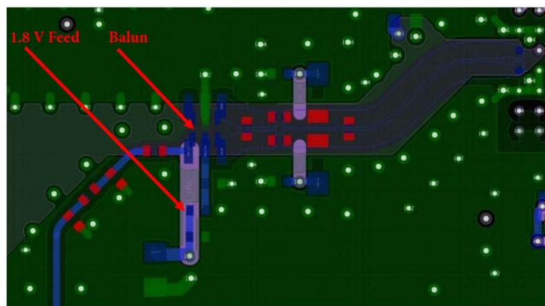
Figure 141. 1.8V TX Bias Routing at Balun
