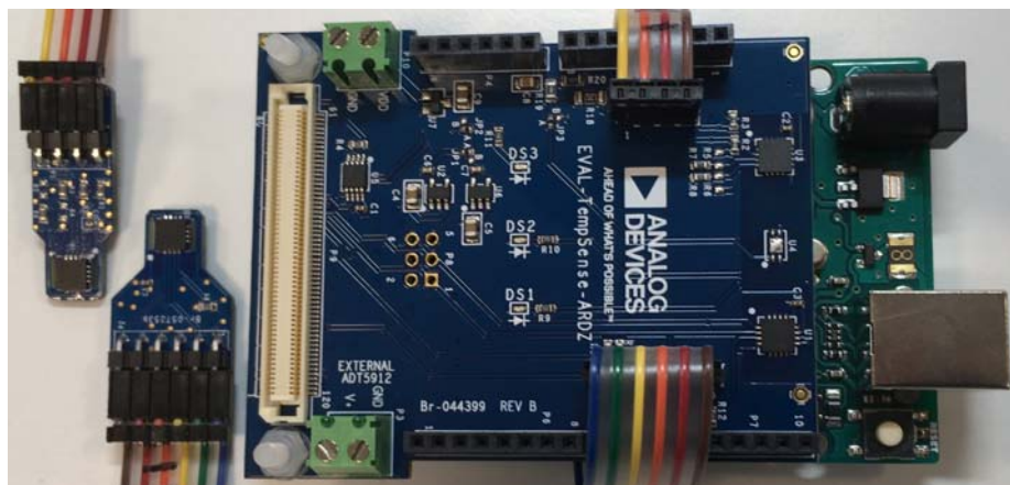
Figure 5. Hardware Connected Diagram
