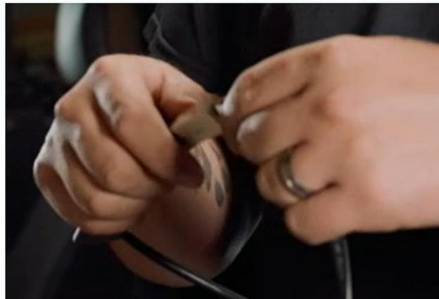
3. Connect the Cat6 shielded Ethernet extension cable to the other end of the RJ45 female coupler.
