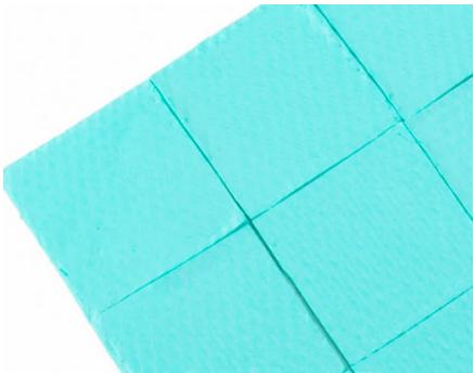
Laird Tflex™ HD80000 is the latest product in the High Deflection gap filler series. Tflex™ HD80000 combines 6 W/mK thermal conductivity with superior pressure versus deflection characteristics. The combination will allow minimal stress on components while also yielding low thermal resistance. As a result, less mechanical and thermal stresses will be experienced within your device.
