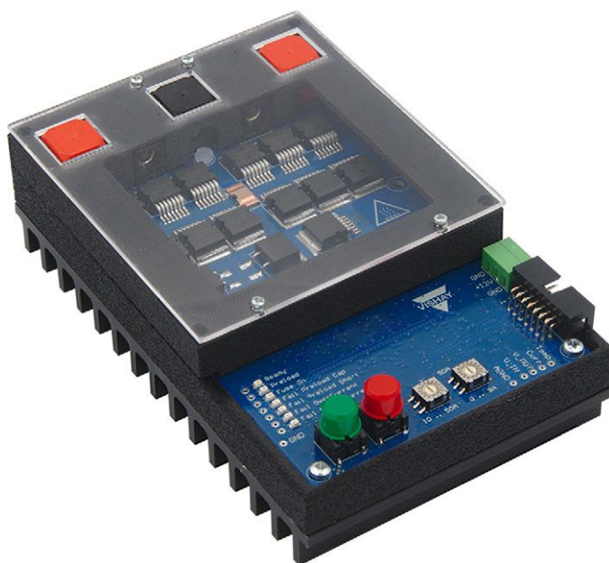
Fig. 19 - eFuse Including Heat Sink and Case
