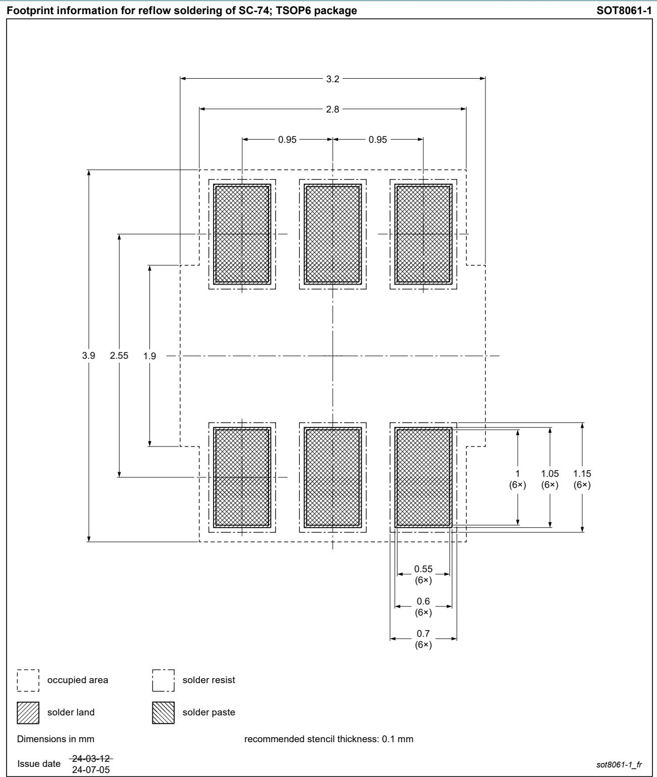
Fig. 2. Reflow soldering footprint for TSOT23-6 (SOT8061-1)
