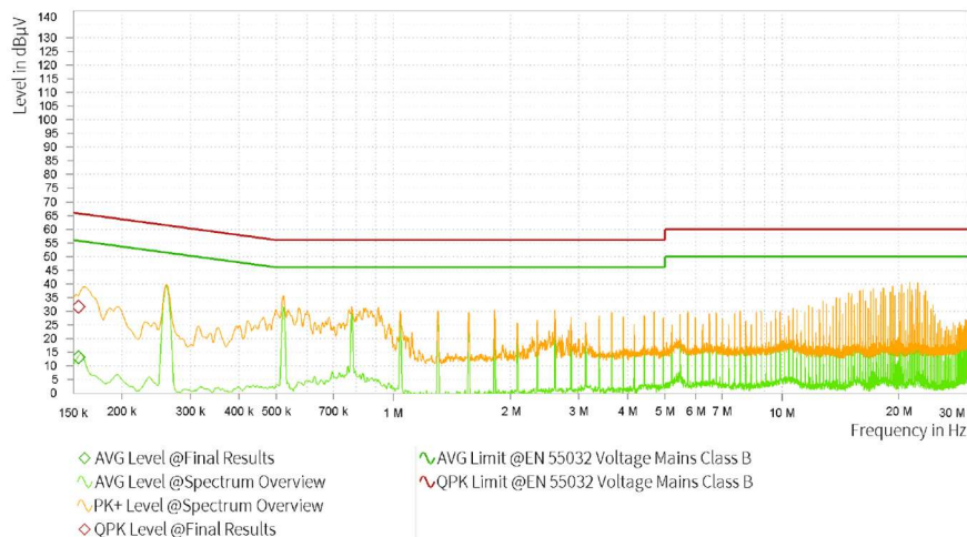
REC10K-2415DAW/H2, 24VIN – EN55032 Class B Emission test
