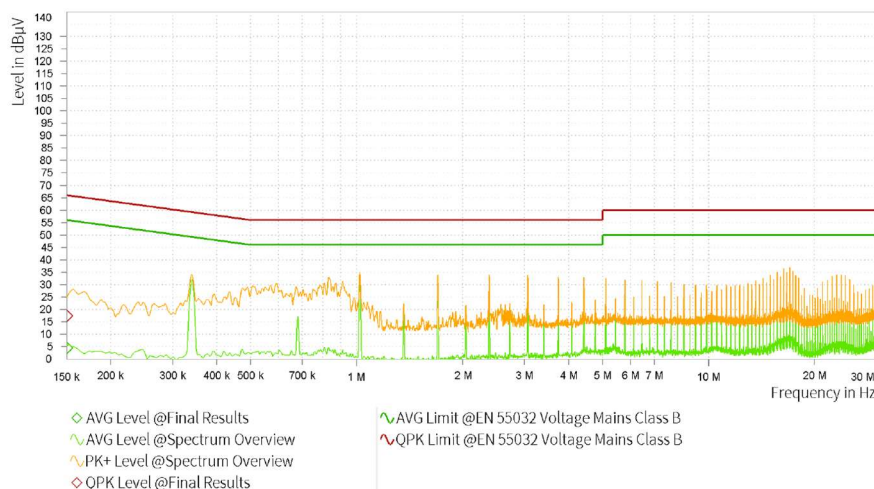
REC10K-4805SAW/H2, 48VIN – EN55032 Class B Emission test
