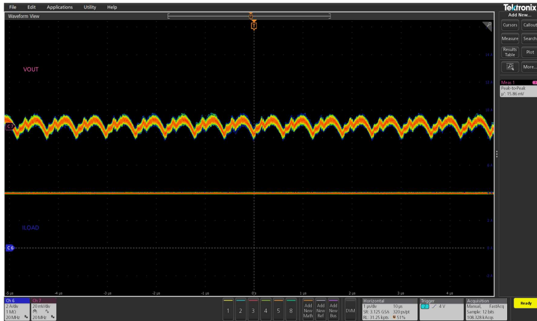
Figure 17 V_{OUT} ripple at 4A (Ch6: I_O , Ch7: V_{OUT} ), Peak-Peak V_{OUT} ripple = 15.9 mV
