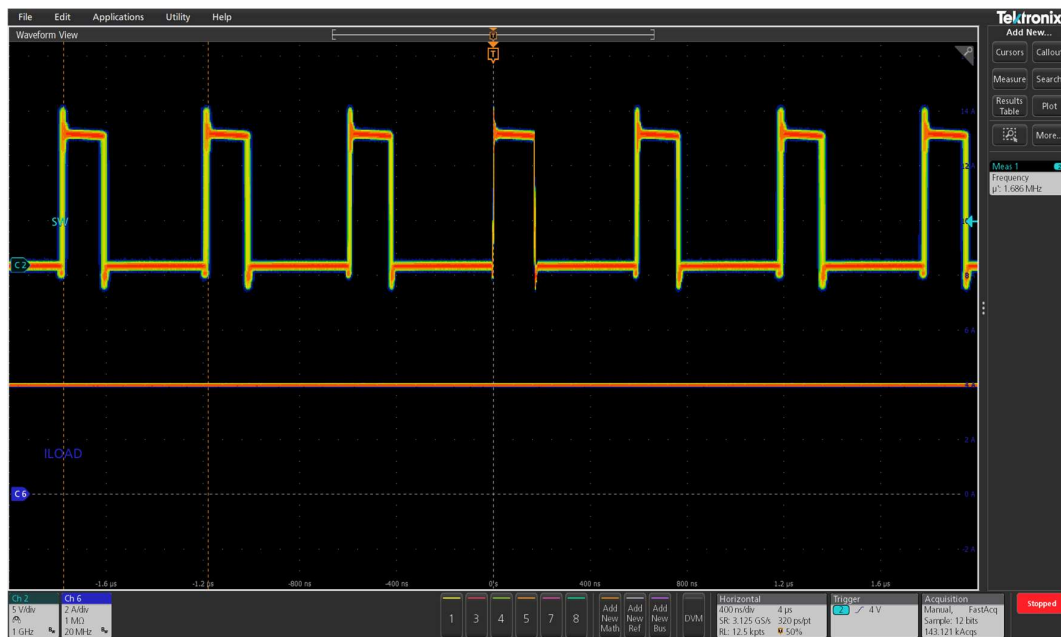
Figure 15 Sw at 4A (Ch2: Sw, Ch6: I_O ), F_{SW} = 1.69 \text{ MHz}
