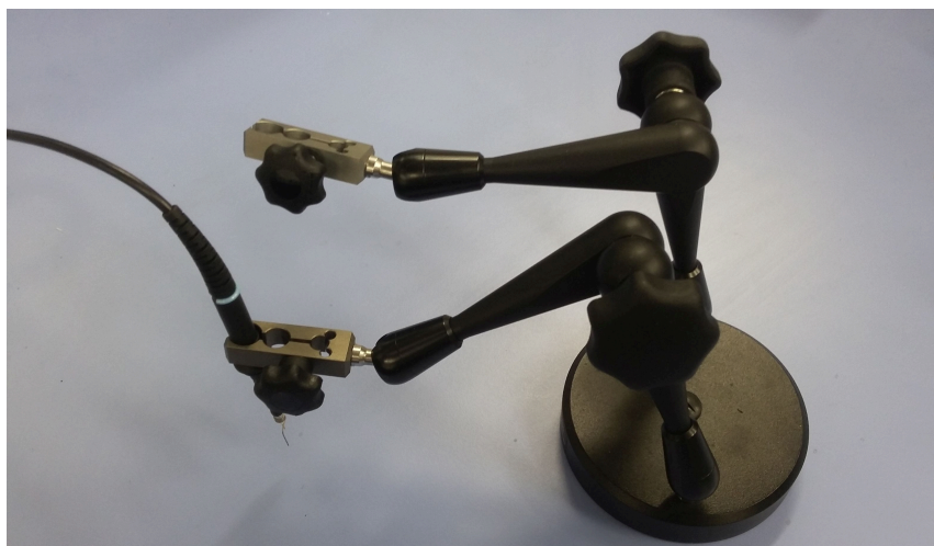
Fig. 2. Example of a probe positioner
