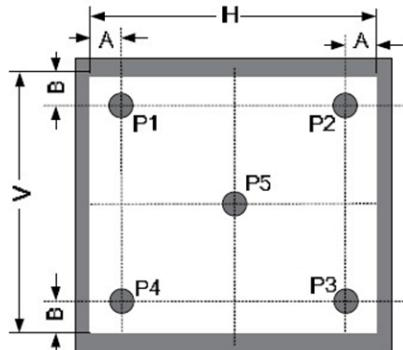
*Measuring method for Contrast ratio, surface luminance,
