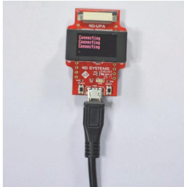
*Connection of an IoD-09TH Display module to 4D-UPA with a micro-USB Cable*
