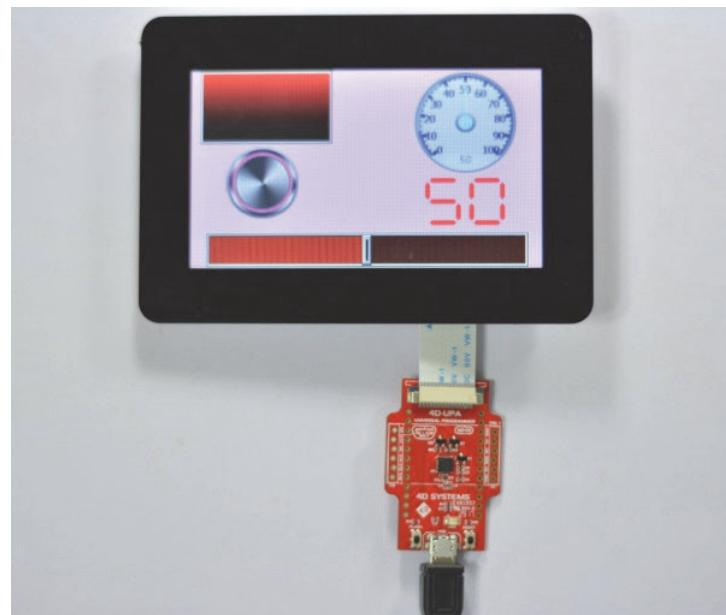
*Typical connection of gen4 display module
