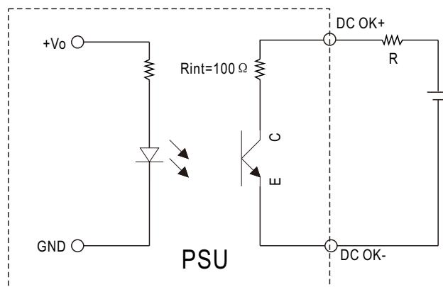
External voltage source(V) and resistor(R)
