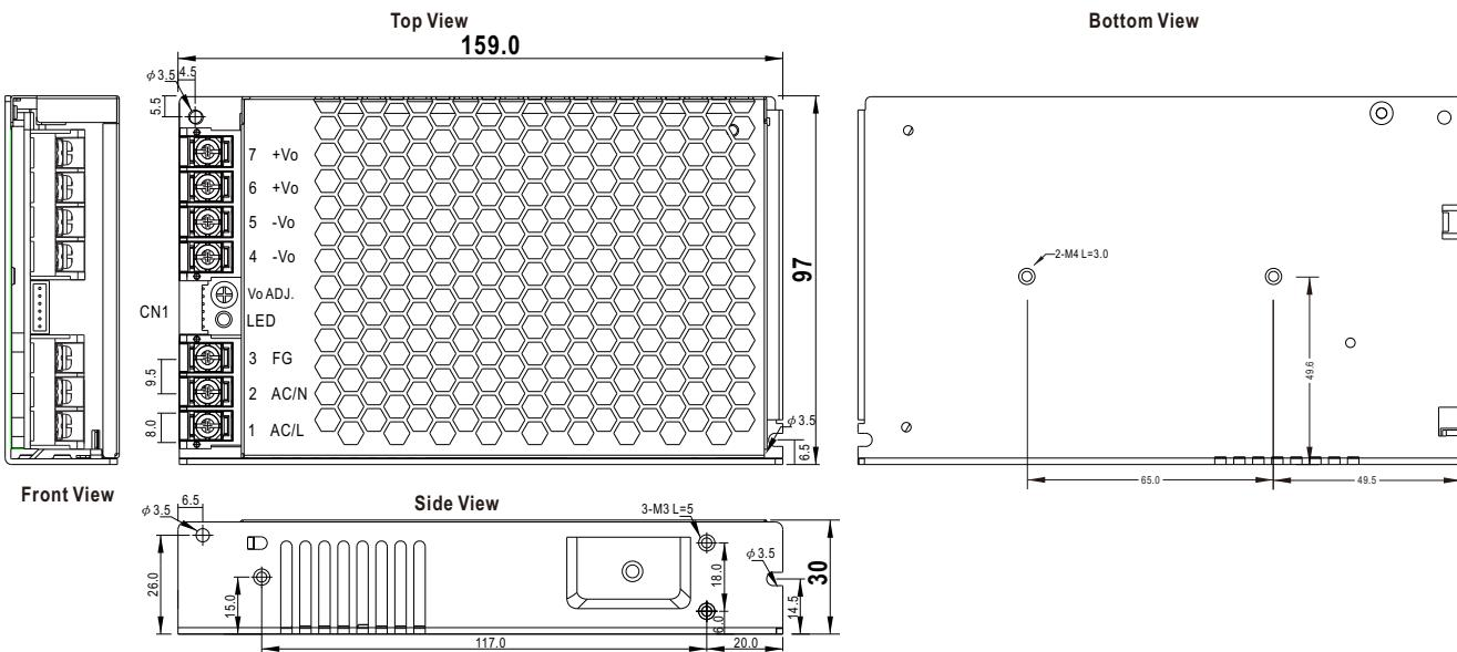
**※ Input Terminal Pin No. Assignment**
