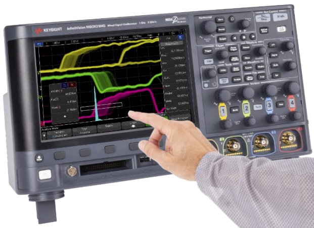
Figure 2. An 8.5" capacitive touch display with large, touchable targets.
