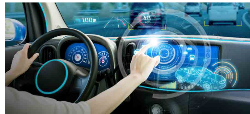
Figure 2: Giant capacitive touch screens featured on newer cars are susceptible to false triggers which can be prevented using a force-sensing home button
