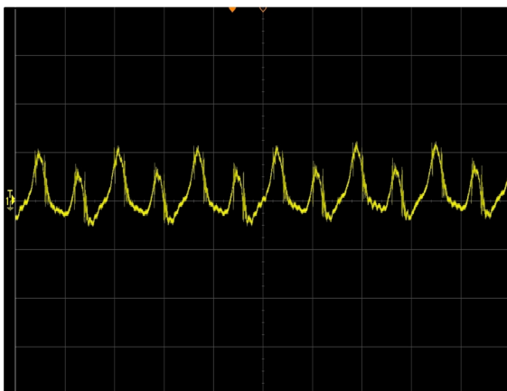
Figure 5: NDQ1300-48S12B-6I Ripple and Noise (5μs/div) Vin = 50V Load: Io = 106A Ch 1: Vo (20mV/div)
