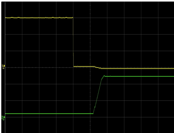
Figure 3: NDQ1300-48S12B-6I Remote On Waveform (50ms/div) Vin = 50V Load: Io = 106A Ch 1: Remote On (1V/div) Ch 2: Vo (5V/div)
