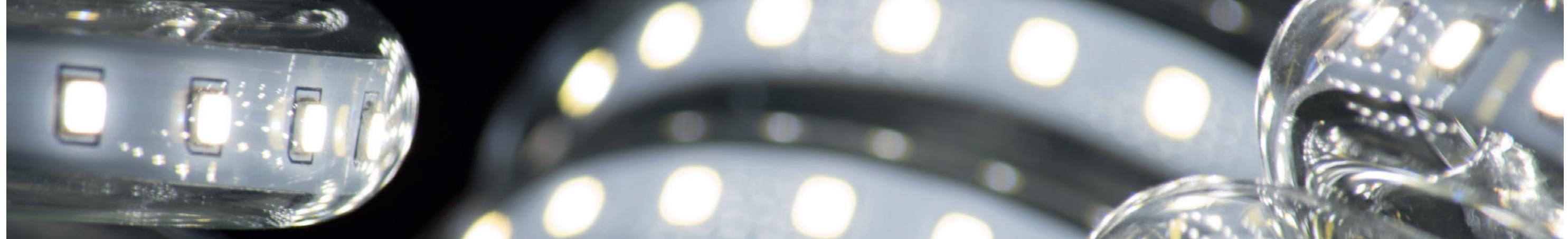
Loads with capacitive load shares, especially LED lamps, place extreme demands on the switching contacts, regardless of the voltage type. They produce extremely high-energy current peaks at the moment of switching on. These can reach over 100 A and weld the contact.
