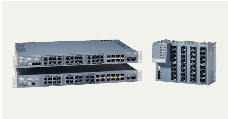
Rack variants with different numbers of ports from the SCALANCE XR-300 or SCALANCE XRM-300 product series (left) and compact switches SCALANCE XC-300 or SCALANCE XCM-300 (right) revolutionize OT networks.
