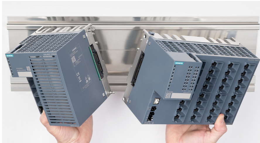
The function extender interface is attached to the right of the SCALANCE LPE processing platform and to the left of the SCALANCE XCM-300 Ethernet switch. This makes it easy to integrate the LPE into the network (the switch) – the devices are mounted on the DIN rail and the connection works without any cabling effort.
