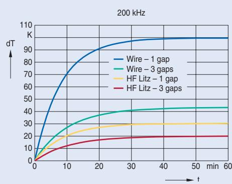
With distributed air gaps, solid wire designs may perform as well as litz wire designs but with a better  $R_{\text{DC}}$ .
