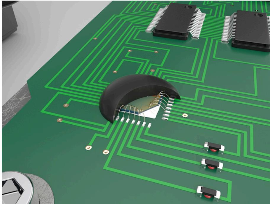
Provides environmental protection and adds mechanical strength to wire bonded devices.
