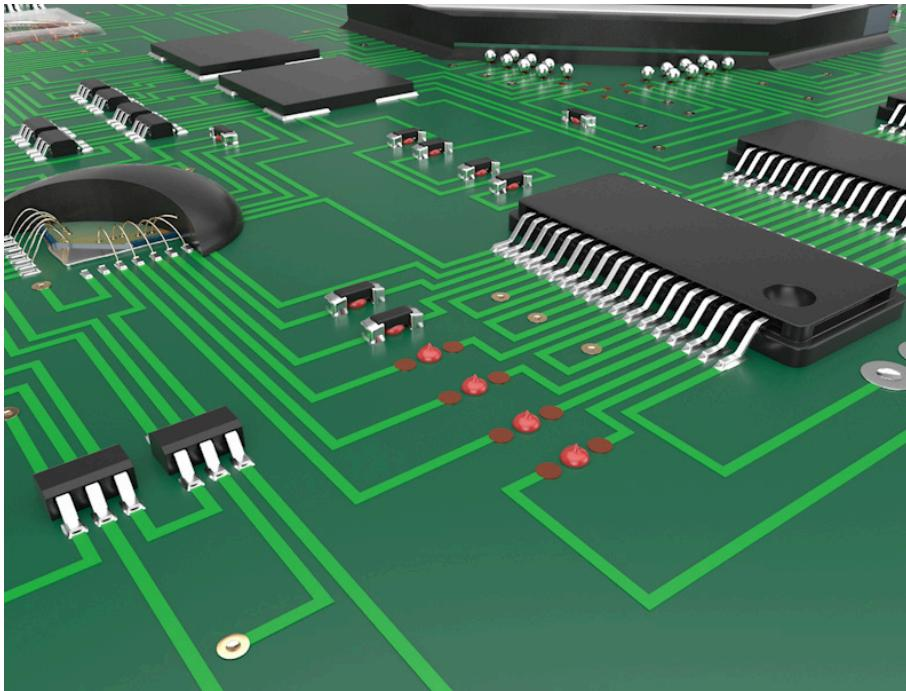
Secures surface mount components in place during the wave soldering process.
