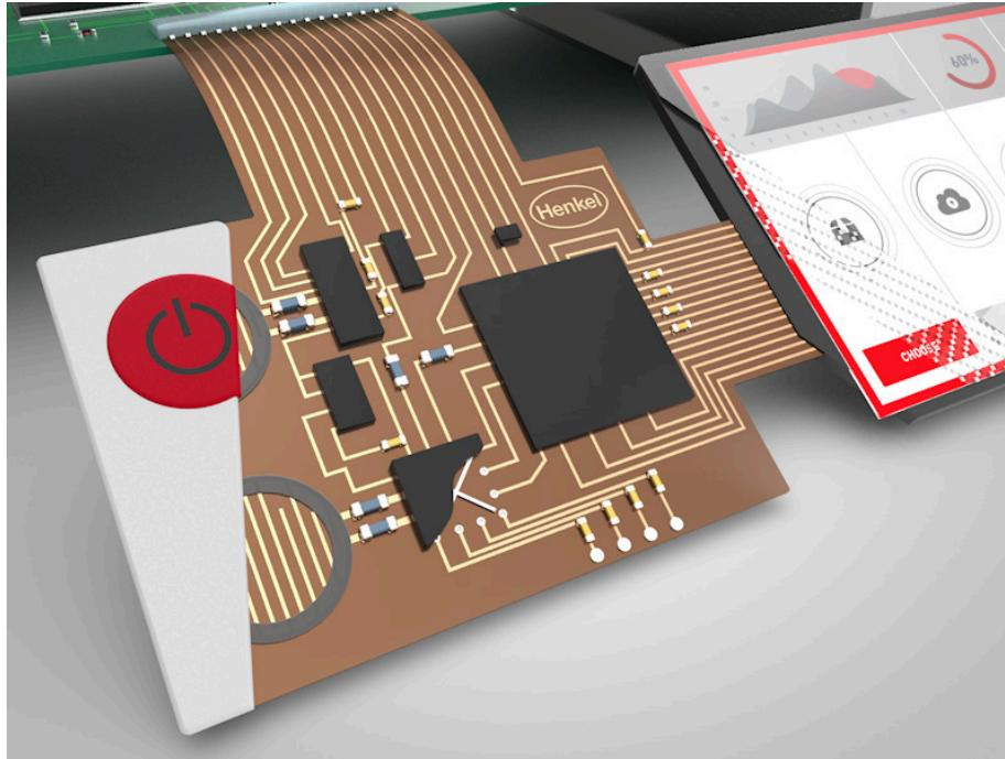
Selectively coats on a variety of flexible and rigid substrates, via screen, flexographic and rotogravure printing methods.
